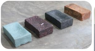
Fig 3: Bricks from Plastic Waste
