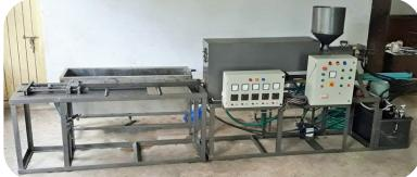
Fig 7: Two stage Extruder-Injection Moulding machine
