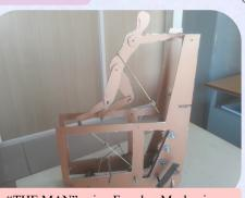
"THE MAN" using Four bar Mechanism
