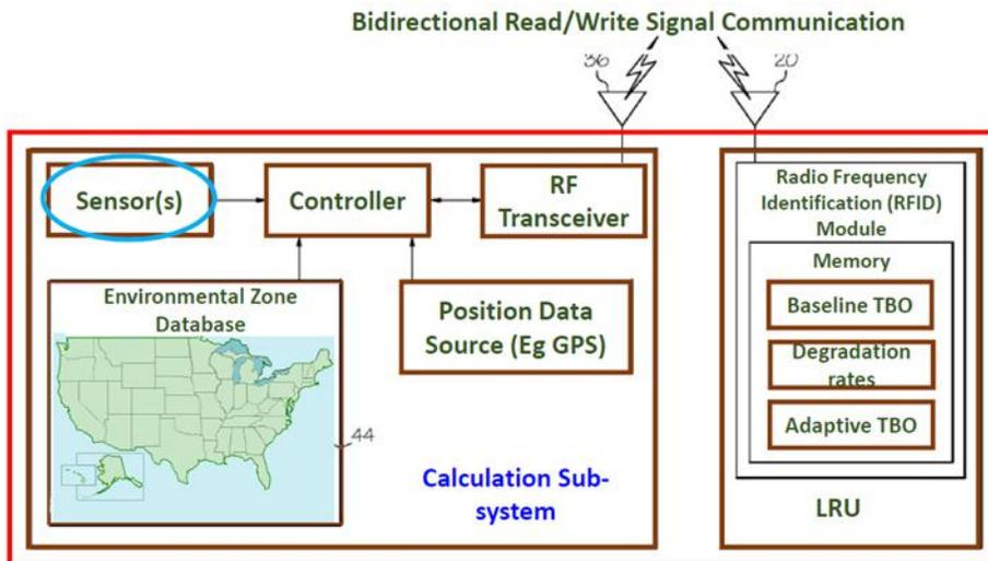
Fig. 1. Line Replaceable Unit Prognostic System
