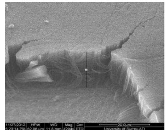
**Fig. 2:** Scanning Electron Microscope image of a VANTA coating grown on an Aluminium Substrate
