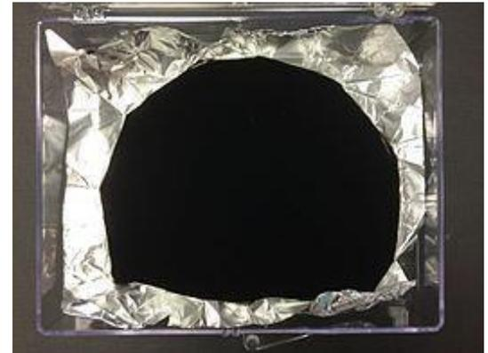
**Fig. 1:** Aluminium foil with a portion coated in Vantablack
