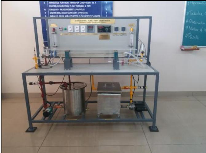
CONCENTRIC TUBE HEAT EXCHANGER
