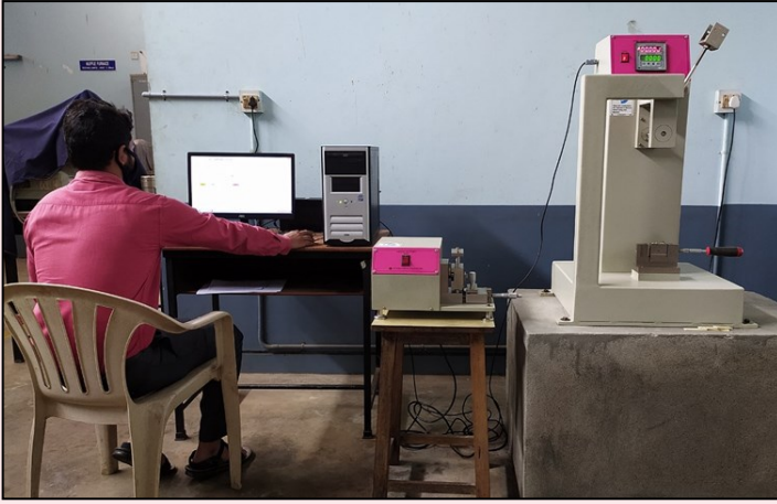
Computerized Impact Testing Machine for Polymers and its Composites (with the motorized notch cutter)
